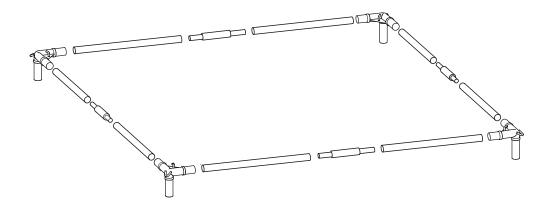
**Step 1**: Lay all the parts on the ground as shown.
