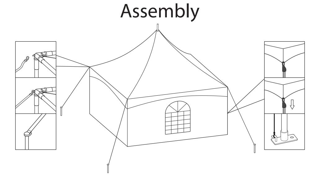
**Step 9**: Fasten the roof tensioning ropes and use the roof tensioning strapes make the tent more stable.
